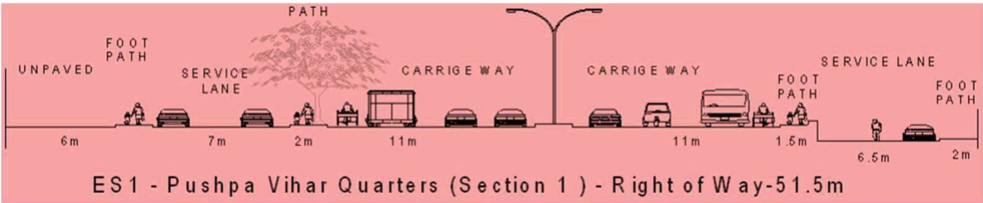
Fig.9a Before BRT road cross section
